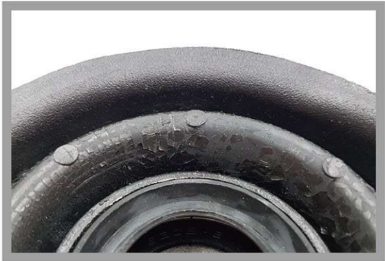
Recycled , low grade rubber causing premature cracks and poor finish.
