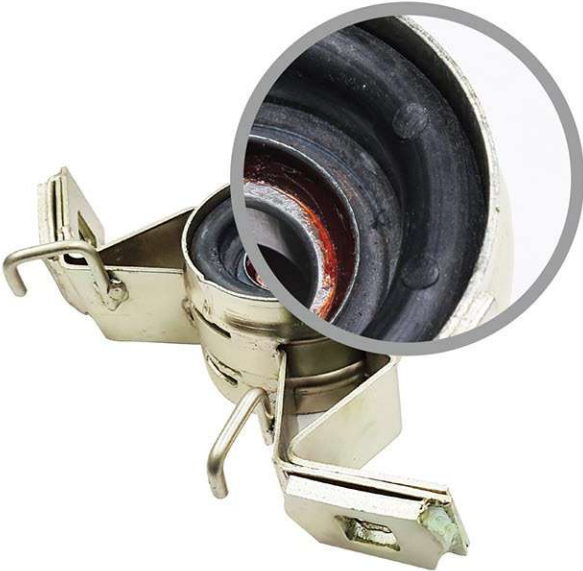
Incorrect rubber to bracket design. Over-stiffed rubber which compromises damping ability.
